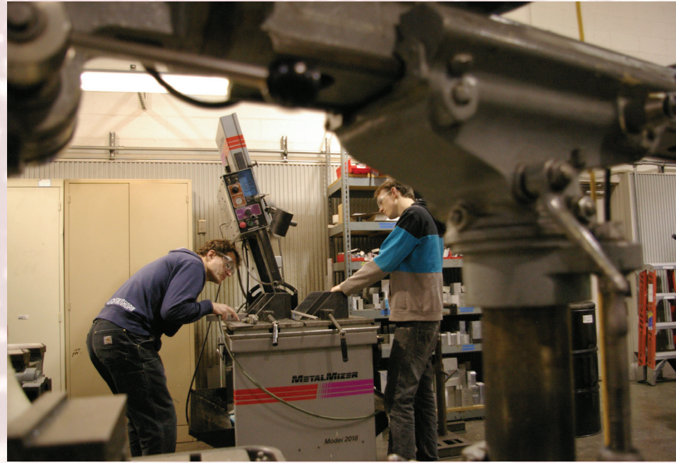
Professor Eric Leonhardt and student Jacob Thurber work with a metal saw to cut an aluminum frame piece for a senior project campus electric vehicle. // Photo by Cody Clark
