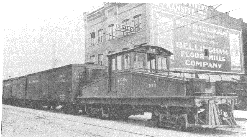
Figure 48. A Whatcom County Railway and Light freight locomotive moving Great Northern cars from the Larson Mill to McKenzie Street. After 1912, this type of freight movement was handled entirely by the interurban line. (Puget Power Collection, CPNS)
