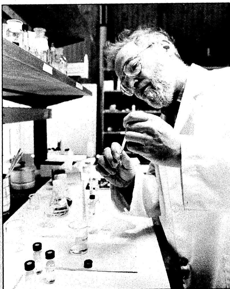
Mayer fills a syringe with diazinon to be injected into the gas chromatograph.
