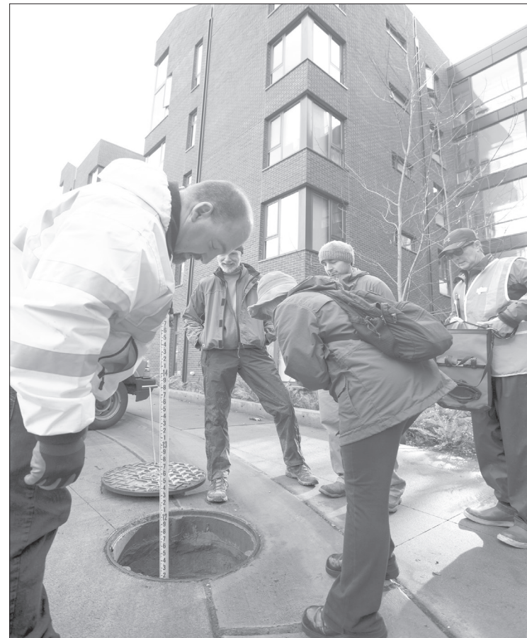
Mark Howard, the stormwater engineering technician for the City of Bellingham, shows the depth of the storm-water holding tank located underneath the parking area directly behind Buchanan Towers East on Saturday, Jan. 16. // Photo by Ian Koppe
