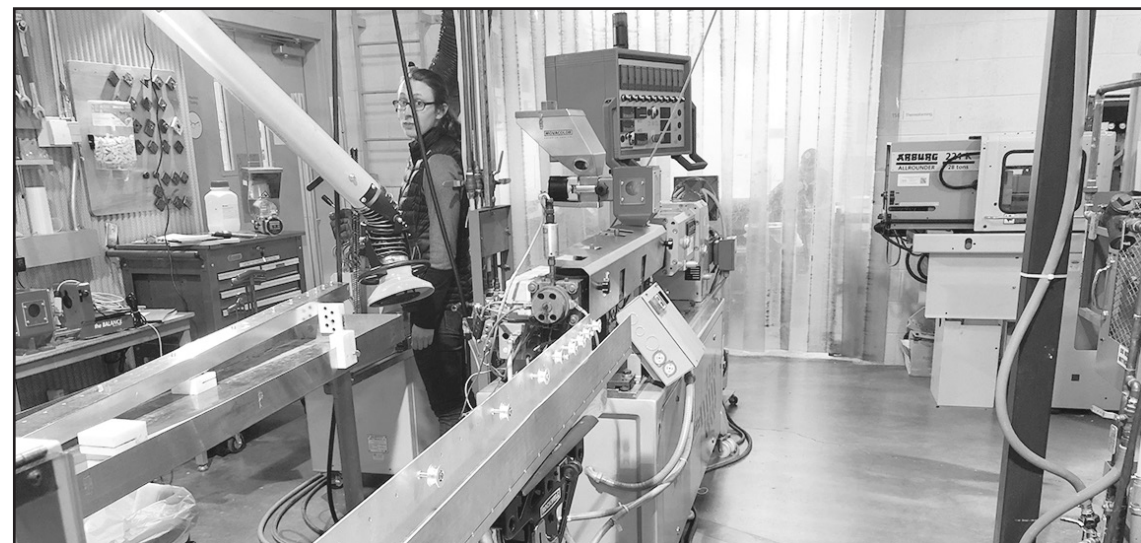
In the production line, non-reusable plastic bottles are turned into usable filament for 3D printers. // Photo by Daniel Lee
