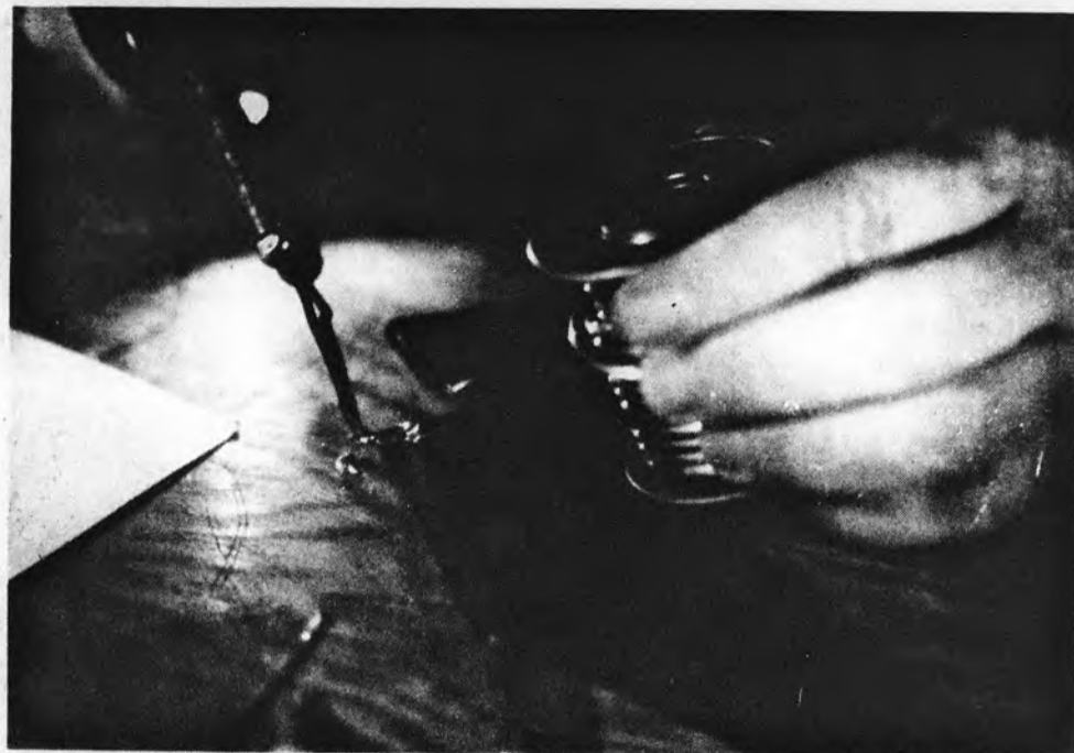
The cane is fitted along the glass pieces, cut to size, and soldered.
